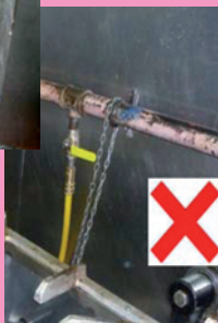
Restraining wire attached to the pipework
