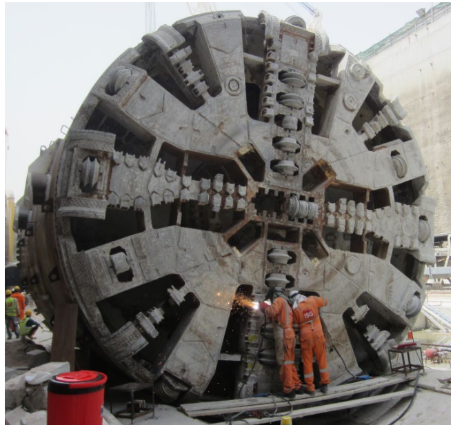
Tunnel boring machine © Vinci
